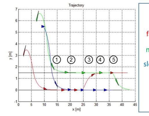
In the presented case: N = 3fast  $[x_1(t_0) \ y_1(t_0) \ \theta_1(t_0) \ \phi_1(t_0)] = [2 \ 3 \ \pi/4 \ 0]^T$ mid  $[x_2(t_0) \ y_2(t_0) \ \theta_2(t_0) \ \phi_2(t_0)] = [7 \ 6 \ \pi/4 \ \pi/4]^T$ slow  $[x_3(t_0) \ y_3(t_0) \ \theta_3(t_0) \ \phi_3(t_0)] = [9 \ 5.5 \ 0 \ 0]^T$   $[s_0(t_0) \ s_{d0}(t_0)]^T = [0 \ 0]^T$  for all virtual vehicles Desired speeds are  $[v_{d1} \ v_{d2} \ v_{d3}]^T = [6 \ 5 \ 4]^T$
