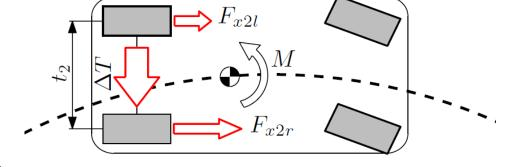
**Electronic differential** (for Electric Vehicles with Independent Motors
