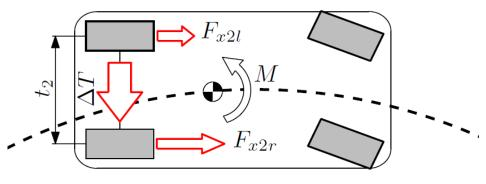
Figure: The function of a rear active differentials.
