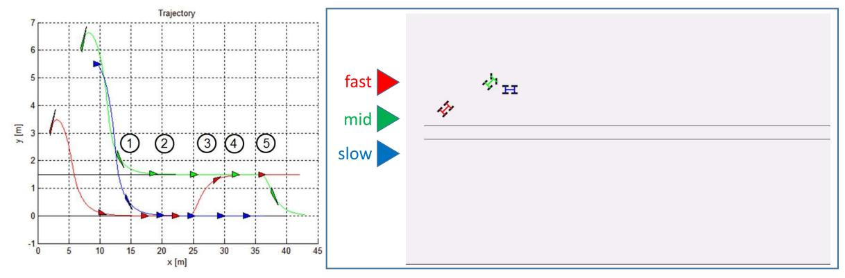
Vehicle length l = 1Safety zone  $[d \ w]^T = [2.5 \ 0.41]^T$  Path following control gains  $\begin{bmatrix} k & a_1 & a_2 \end{bmatrix}^T = \begin{bmatrix} 2 & 2 & 4 \end{bmatrix}^T$ Coordination control gains  $\begin{bmatrix} \lambda & \gamma_1 & \gamma_2 \end{bmatrix}^T = \begin{bmatrix} 0.2 & 0.5 & 0.5 \end{bmatrix}^T$
